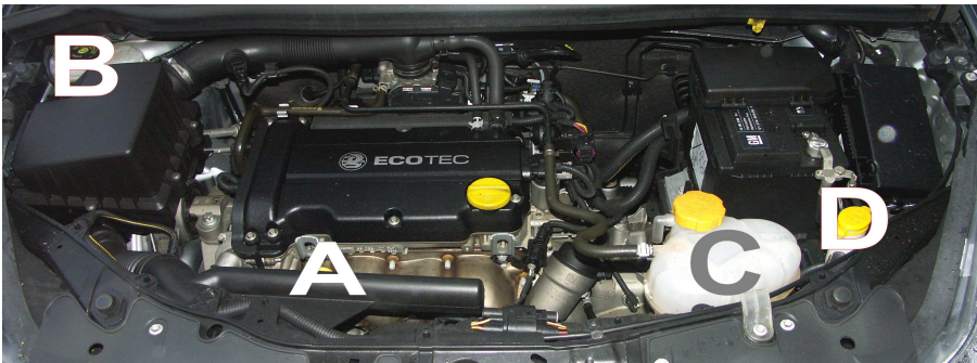
A = Dipstick B= Brake Fluid Reservoir C= Coolant D= Washer Reservoir
